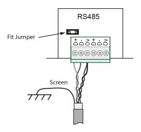
**Note:** The USB/RS485 converter also has a terminating resistor jumper. Ensure that this jumper is always fitted unless the converter has been cabled as an intermediate device in the chain.
