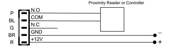
**Note:** When connecting the device to the 'Free Exit' input of an access control unit, we recommend that you set the latch time to the same value as that set in the access control unit so that the LED colour correctly reflects the lock status.
