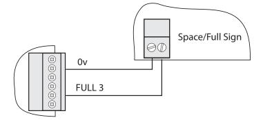
Where the output is used to drive a third party device, it should be wired to the device as shown here:
