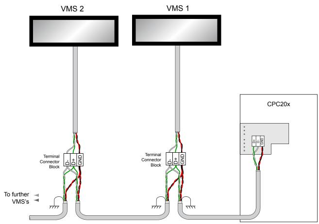
Ground one end of each section of shield as shown
