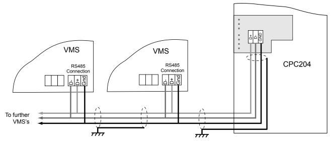
Ground one end of each section of shield as shown
