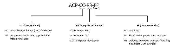
Example: ACP-00-01-01 is a card capture pedestal fitted with a CRC200+ control panel, integral Nortech ISO card reader and Aiphon slave intercom.
