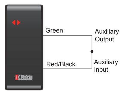
The procedure described in section 6.1 can then be followed to arm and disarm the NanoQuest using an Auxiliary card.
