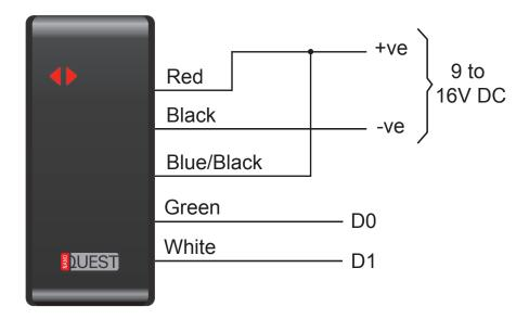
The unit must be powered down, rewired and then powered up again. The standalone functions are no longer supported and, when a card is presented, it simply reads the card and forwards the card number to the external access controller.
