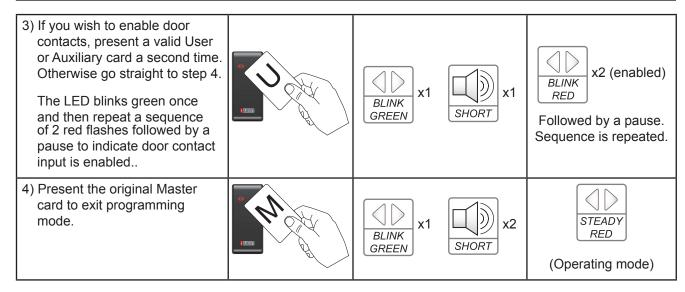
While in 'Use Door Contact' mode, if you do not present any cards for a period of thirty seconds, the NanoQuest will exit programming mode and return to normal operation.
